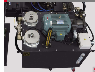
Picture shows 70BAR coolant supply unit OP
