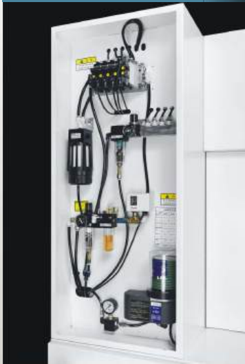
Pneumatic and Lubricant system
