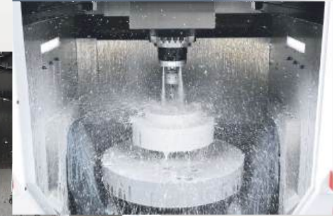
Circular water Flushing System
