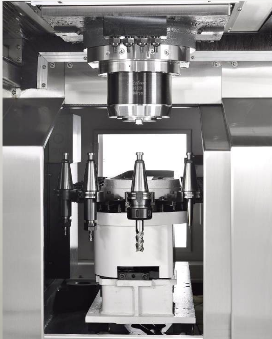
■ The Dual-Magazine Unit is designed for option by the customer according to different workpiece and demand for the number of Tools.
