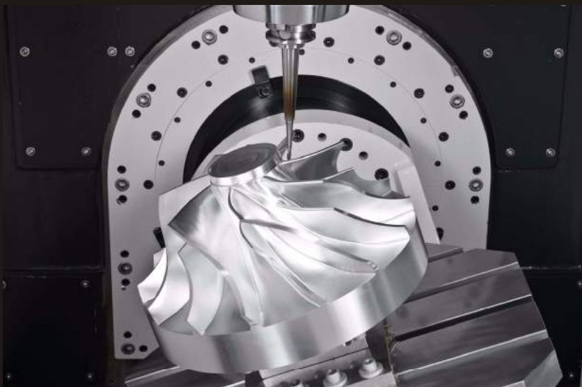
Highly efficient 5 axes machining application.
