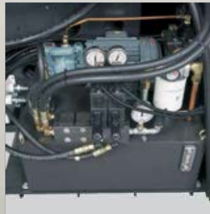
Worktable Hydraulic Brake Unit
